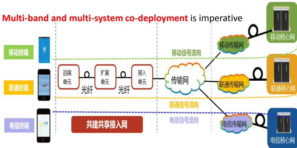
In the 2G/3G period, the main forms of coverage are outdoor macro base stations and indoor DAS. However, with the explosive growth of data traffic in the later 4G network and the gradual increase of the frequency of 5G base stations, the coverage of single base station decreases, **the operators are paying more and more attention to the small cell products. Facing 5G, digital indoor coverage will gradually become the new standard for indoor network construction.**
